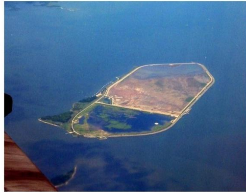
Figure 3.1-13: Example of a Confined Disposal Facility (CDF)
